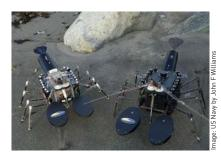
Robo-Lobster is a biomimetic underwater autonomous robot designed to move in shallow water just like a real lobster. It uses an electronic nervous system which is programmed to behave the way a lobster does as it searches its environment.
