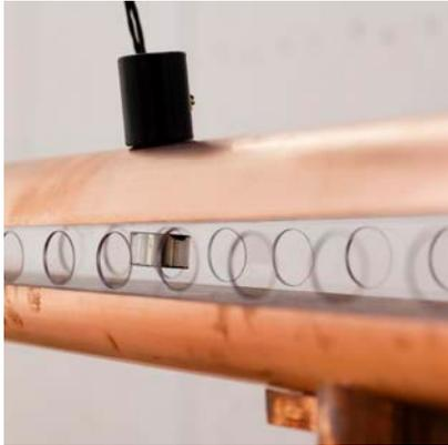
Floating Magnet shows eddy currents, which are created because of the close relationship between electricity and magnetism. Eddy currents are circular electric currents that are induced inside a conductor by a moving magnet.
