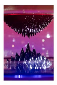
Magnetic Liquid contains a special material called a ferrofluid, which has some interesting properties. Ferrofluids are made from magnetic material that has been ground into an extremely fine powder and suspended in a liquid. This effectively means that the magnetic particles are evenly distributed throughout the liquid, giving it an overall magnetic property.
